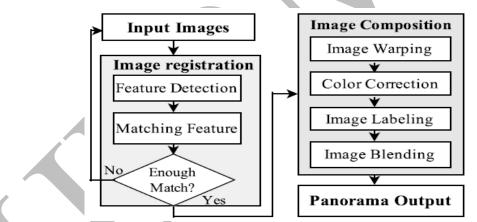
Fig. 1 The block diagram of general panorama image stitching model based on feature based approaches
